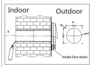
4. Paste the location sticker on the wall surface. Pay Attention to the direction to make sure the circle on location sticker and duct to be concentric. Marking the drilling hole site and remove the location sticker. Drilling 4\*6mm hole on the marking place and put in the rubber plug(as pack accessories)
