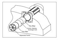
6. Install the ventilation unit on the mounting plate. The ventilation unit is fixed with magnets.
